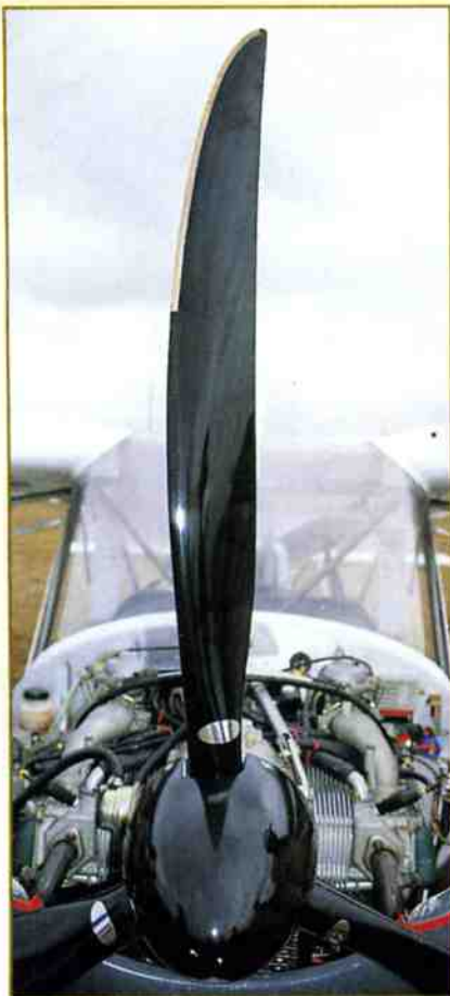
The magnificently efficient Kiev propeller. The curved blades add quietness.
