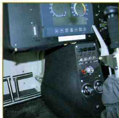
The control stick is substantial, but neat and comfortable in operation. The brake pedals are well made. Single brake on the stick works just fine. Note the Brauniger "glass cockpit" above the businesslike center console.
