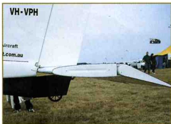
Tail surfaces are separate. Note the wheel to stop the tail bumping when lifting the nose during ground handling.
