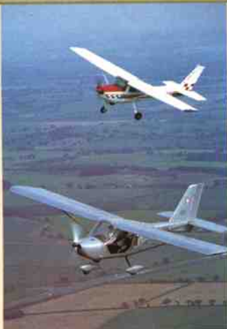
Foxbat's fuel burn is around half the 152's five gallons an hour
