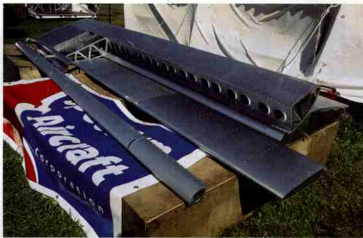
The riveted wing's main spar is positioned 13.5 inches behind the leading edge and is built up as an I-beam and extruded angle caps.
