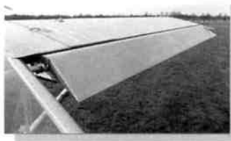
Full-span flaperons give ample roll authority.
