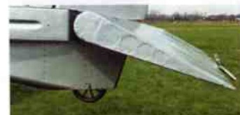
Neat semi-recessed tailwheel.
