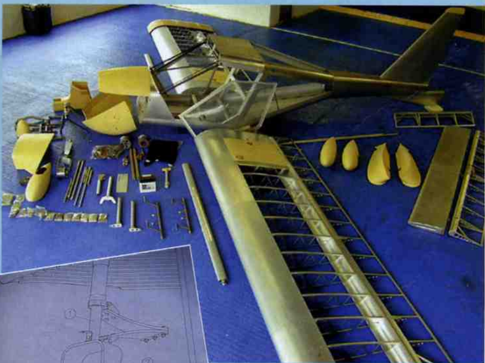
Above: the fuselage, wings, tailplane, fin and all control surfaces come pre-ripped.
