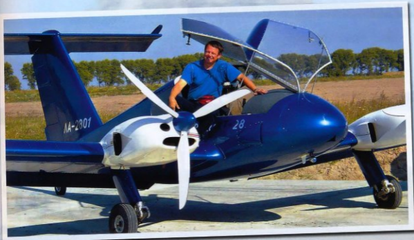
Above: Yuri Yakovlev and another of his innovative designs, the Aeroprakt A-28, powered by a pair of Rotax 912 engines.
