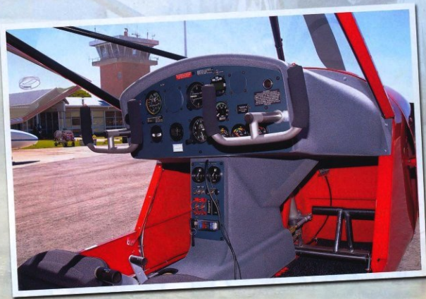
Aeroprakt gambled on the extra expense of a yoke option - it has been a popular and unusual (for a VLA) choice.
